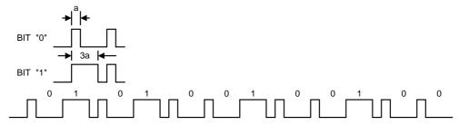
One word of the above transmission command is in the configuration of (010100100100).
